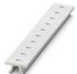
Zack marker strip, Strip, white, labeled, can be labeled with: CMS-P1-PLOTTER, printed horizontally: Identical numbers 1 or 2, etc. up to 100, mounting type: snap into tall marker groove, for terminal block width: 6.2 mm, lettering field size: 6.15 x 10.5 mm, Number of individual labels: 10
