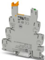
6.2 mm PLC basic terminal block with screw connection, without relay or solid-state relay, for mounting on DIN rail NS 35/7,5, 1 changeover contact, input voltage 5 V DC
