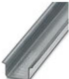
DIN rail, unperforated, Standard profile, width: 35 mm, height: 15 mm, similar to EN 60715, material: Steel, galvanized, length: 2000 mm, color: silver
