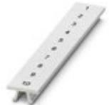
Zack marker strip, Strip, white, labeled, can be labeled with: CMS-P1-PLOTTER, Printed vertically: consecutive numbers 1 ... 10, 11 ... 20, etc. up to 491 ... 500, mounting type: snap into tall marker groove, for terminal block width: 6.2 mm, lettering field size: 6.15 x 10.5 mm, Number of individual labels: 10
